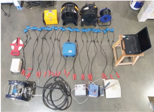
MASW setup with 24-channel seismograph to measure in-situ shear wave velocity
