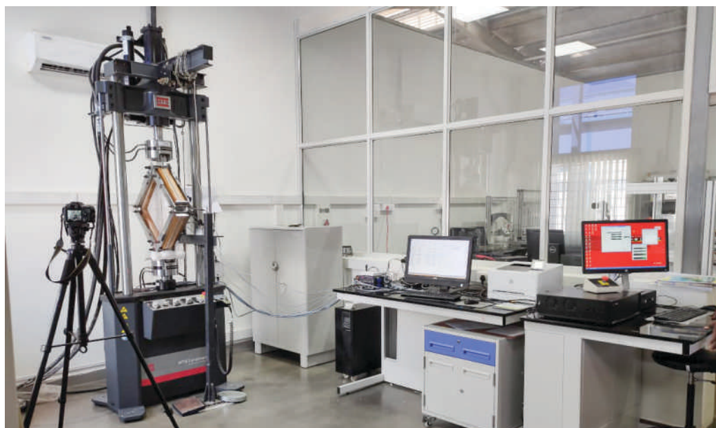
A view of lab with 100kN UTM and DAQ system
