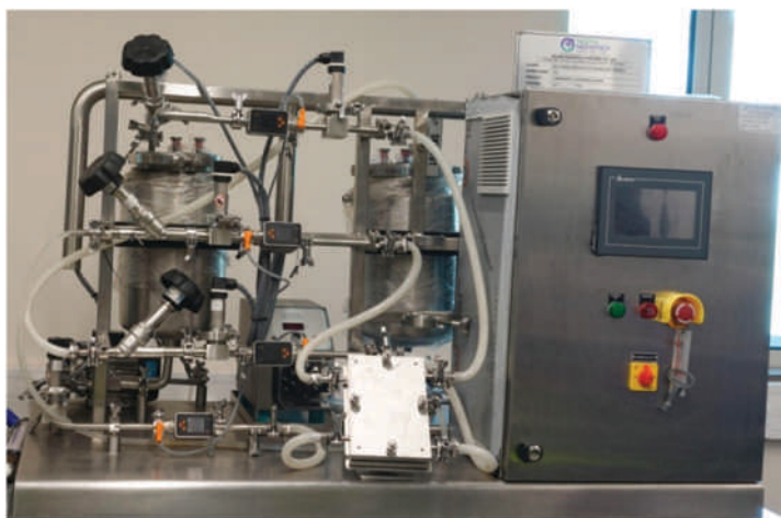
Membrane Systems (NF/RO/OMD)
